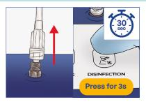
**STEP 3:** Disconnect the disinfectant hose and press the DISINFECTION button for at least 3 seconds.
