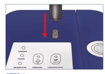
**STEP 5:** Place the disinfected cap on the inlet port.
