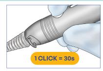
**STEP 3:** Press the handpiece button once to start a 30 seconds cycle. (See IFU for operating modes).
