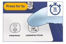
**STEP 2:** Press the DISINFECTION BUTTON for at least 3 seconds. Wait 15 minutes.
