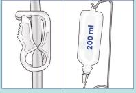
STEP 3: Check if the reservoir contains at least 200 ml of solution. Otherwise replace it.
